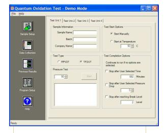
The software package provides automated pressure and temperature monitoring and end point detection for up to four independent *Quantum*™ units. End of test criteria can be selected by Time Duration, Pressure Drop or Break level. DAQ acquisition with USB interface to included laptop...
