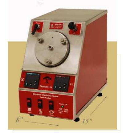
Hot oil baths of varying sizes have long been used in the industry for running the Rotating Pressure Vessel Oxidation Test or RPVOT (formerly known as RBOT) and the Thin-Film Oxygen Uptake test (TFOUT). These bath types expose the operator to hot oil fumes, are prone to leak, need regular maintenance and are generally messy and potentially hazardous to operate.
